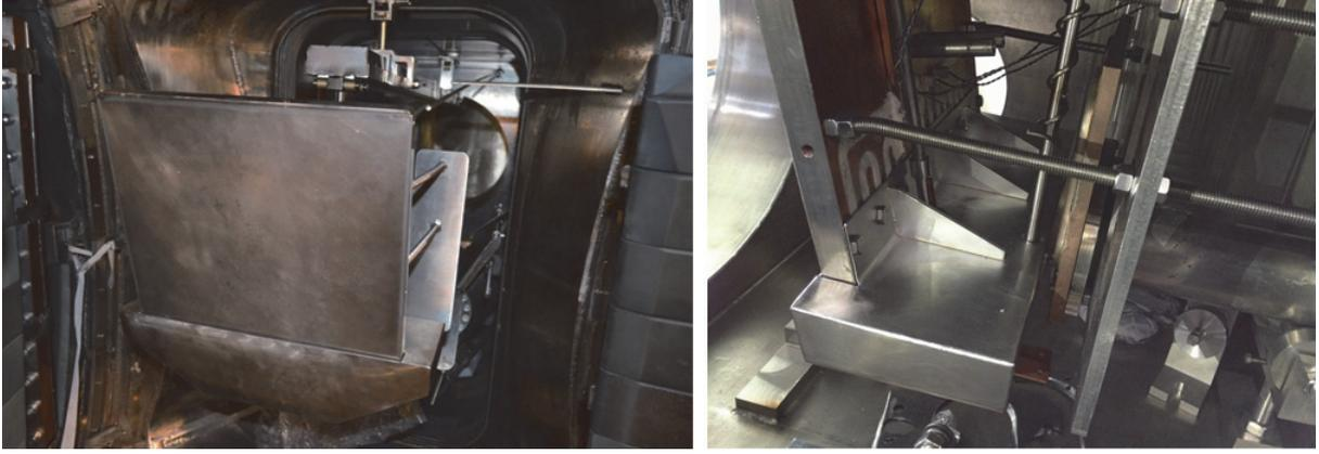
FIG. 4. Two views of the EAST FLiLi limiter assembly. On the left the un-wetted limiter is shown inserted into the EAST vacuum vessel. On the right the limiter is shown in the MAPES exchange box during assembly. The Li supply feed tube is shown inserted into the inlet hole on top of the collector.
