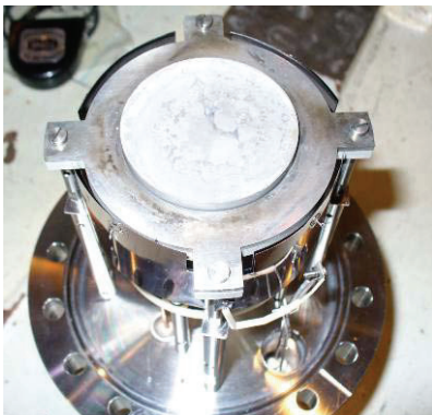
Fig. 1. The electron beam heated ion source with a 50 mm porous tungsten disk and a molybdenum holder.
