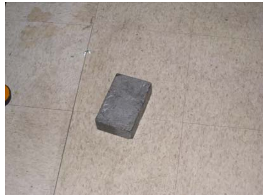
Fig. 11. A block of lead without coating on the floor.
