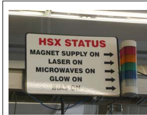
Fig. 29. Information of machine status by colored lights.
